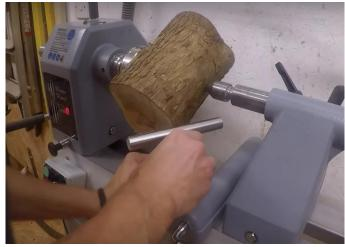
You might think of this as the can of wood (the log) being mounted the wrong way on the lathe.
