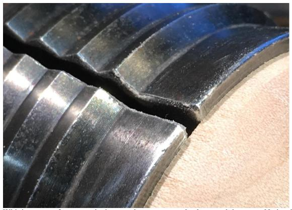
With just over a 2mm gap, the jaws made contact completely around the tenon. Notice the ridge at the base of the jaws in the previous photo is quite uniform from even pressure around the tenon.
