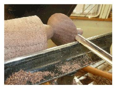
This shows the position of the gouge when cutting the underside of the top surface. Be very careful. If you come in at the wrong angle, you'll chew up the edge and possibly rip off the final. The object is a nice sharp edge. KEEP YOUR FINGERS AWAY FROM the wood...the edges are (or should be) sharp.
