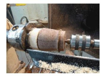
The box has been reversed turned onto a jam chuck for the final shaping of the outside.
