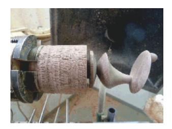
Do the final shaping, sand, and cut off. To part off, I use a parting tool to go down to about 1/4", then stop and use a small saw to cut it off.
