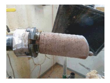
Now the wood is re-chucked on a different axis...opposite of what it was. When you position your tool rest, give the wood a spin by hand to make sure it the wood doesn't hit it. But get it as close as possible. When the wood is away, there will be quite a gap...but almost no gap when it's close. CHECK FIRST before turning on the lathe or you'll get a nasty surprise.
