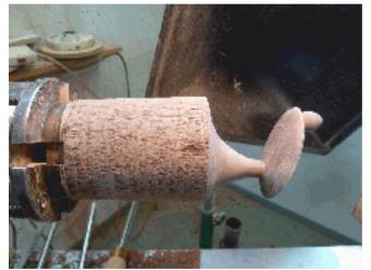
Now the piece had been re-chucked such that's it's in it's normal position. Part down to where you want the lid to start, and make the shoulder that will sit into the base.
