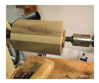
Round the glued-up unit and put tenons on both ends if you are planning a lidded box.
