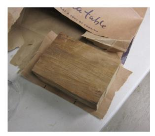
Cut pieces from a brown paper bag slightly larger than the wood block gluing surfaces.
