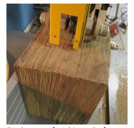
Find a sacrificial board of wood 3/4 to 1 inch thick and approximately the same size as the blocks. Orient the grain of this board the same way as the grain of the blocks. This should be a hardwood not prone to splitting and should not be twisted or cupped.
