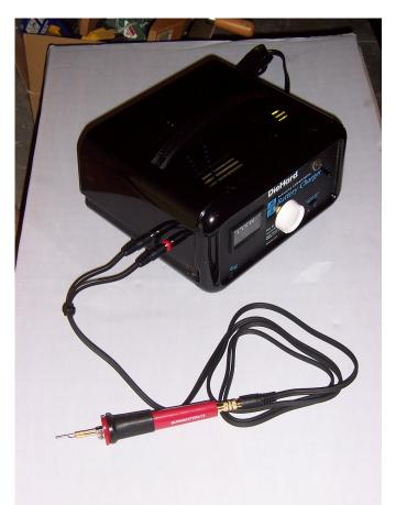
I also tried a ready made cord from Radio Shack and couldn't get the tip to heat up. The cord got warm enough to make a great hand warmer on a cold night but used up too many watts before the power got to the tip. Using the left over battery charger wire and more tips from the Shack, I now can turn the tip bright cherry red in milliseconds. I had the rheostat turned up too high when I plugged it in and almost melted the tip. The charger has a 2 amp and a 10 amp setting, the 2 amp is plenty.
