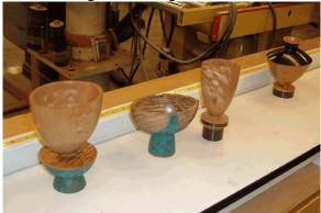
Bill explained how to glue the blank sections with a paper separating the pieces to allow deconstructing the turning without damaging the form. The paper forms a weak joint to the turned sections that is broken with a knife or chisel. The alignment of the blank sections is critical to have the remaining pieces fir properly when reassembling the new shape.
