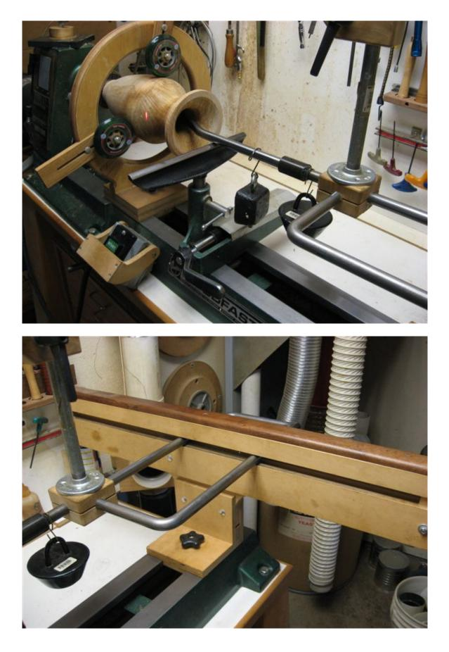
Glenn's photo also shows his homemade laser holder. It's simple and works well. Mine is not so simple and also works well. If anyone would like more details, feel free to contact me with questions or we can schedule a visit to see mine set up on my lathe. I suspect Glenn will be as generous with information about his system.
