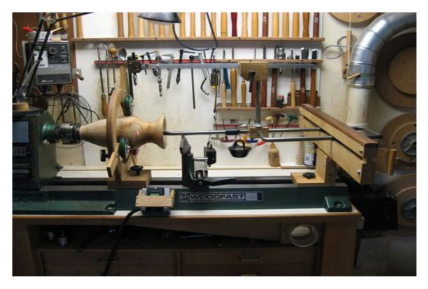
As you can see in the picture, the Jamieson D handle allows for a depth of close to 2 feet. Several of us have made bars that are longer. It's entirely up to the user. If you've never done this, two feet deep is challenging enough, so starting with the Jamieson handle won't limit your turning for the first few years.
