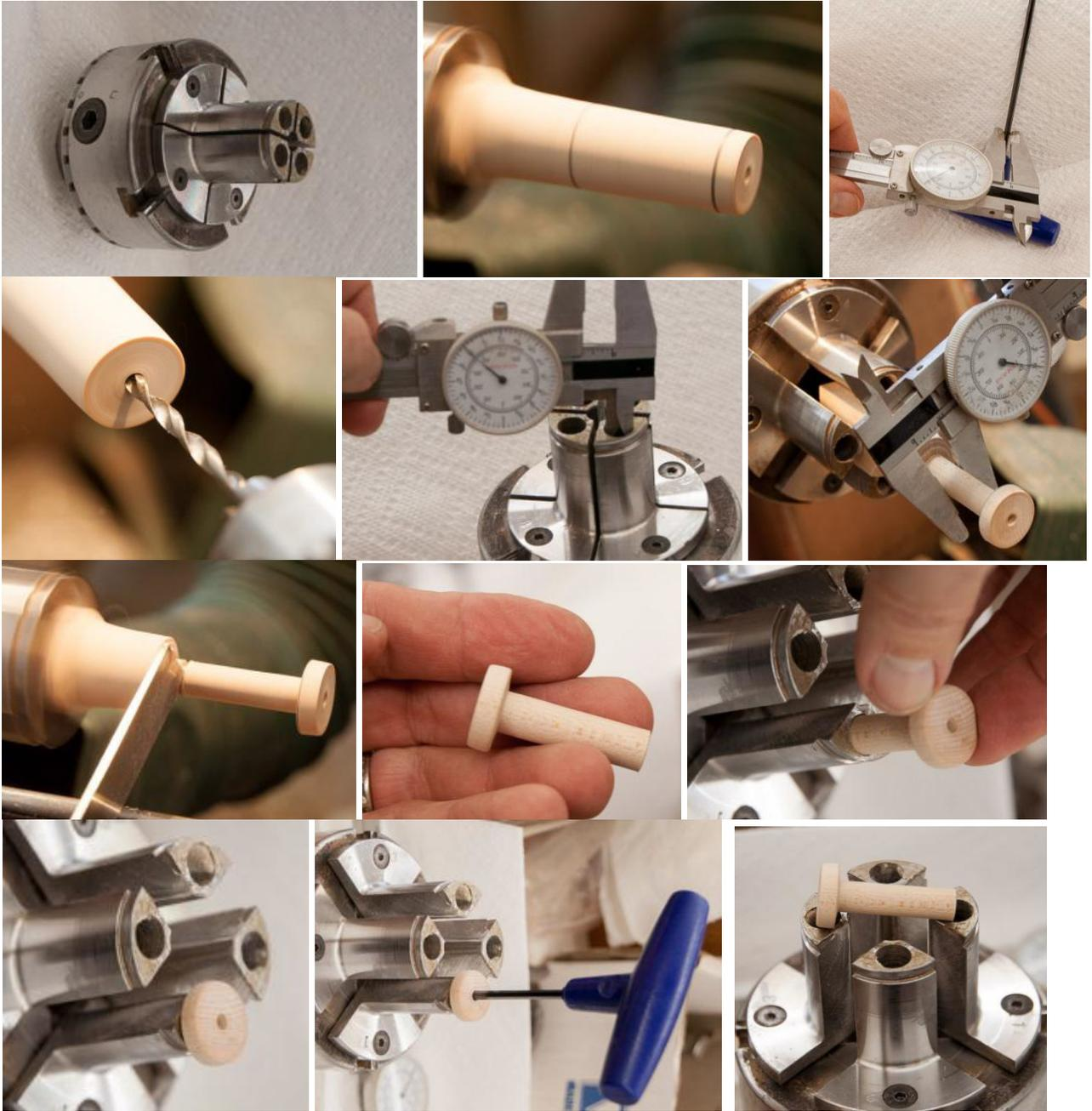
To use the fixture, I simply insert it into the deep hole until the cap is seated, and then insert the 3mm hex wrench, and finding the 3mm hex recess in the mounting screw is a snap. No more frustration!
