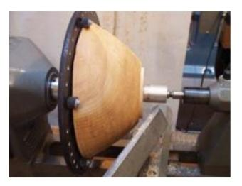
Using a Rim chuck to turn the foot of my rough turned bowl. With the foot turned to fit into the chuck, I mounted the bowl in the chuck and final turned the outside and the inside. Incidentally, I used the cup-shaped live center to support the bowl in the Nova Chuck also. This allows more aggressive turning without concern of losing the bowl from the chuck.
