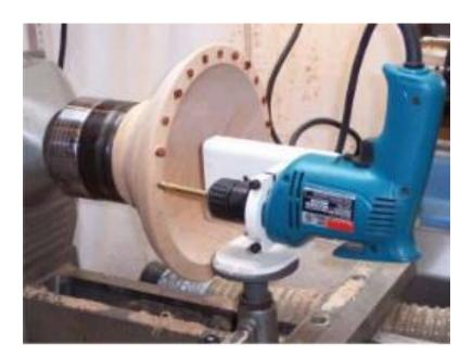
Drilling the 24 equally-spaced holes with the Oneway Drill Wizard and my 3/8" drive drill motor that had to be purchased to fit the collar of the Drill Wizard.
